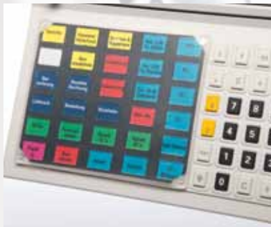
Silicon membrane panel with 30 keys
